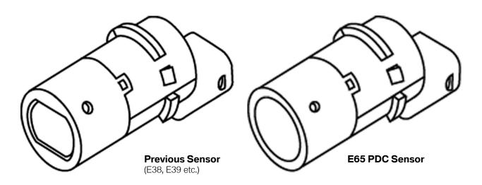
The advantages of this new round membrane shape are the greater detection range and lower sensitivity in wet conditions. The sensors are always painted in body color.
